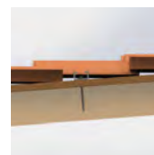
4. Screw the 5/16" lag bolt into rafter, embedded min. 2.5" tightening torque depends on the planned location.
