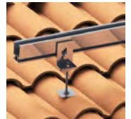
9. Attach rail to the headless threaded bolt using two 3/8" nuts.
