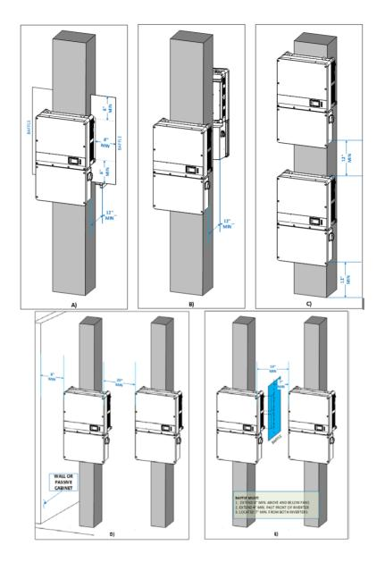
Figure 2.4 - Inverter Pillar Mounting Specifications
