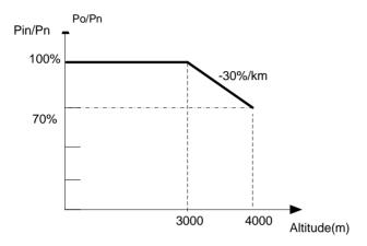
Figure 7.4 - PVI 50/60TL Derating Curve with High Altitude
