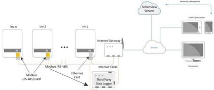
Figure 2.43 - PVI 50/60TL Inverters in a RS-485 Daisy Chain Connection to an External DAS
