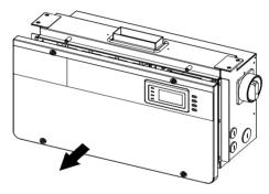
Figure 2.34 - Remove the Wiring Box Cover
