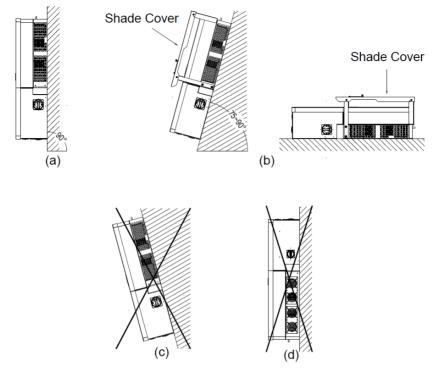
Figure 2.2 - Inverter Mounting
