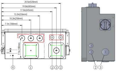
Figure 2.20 - External Connection Ports
