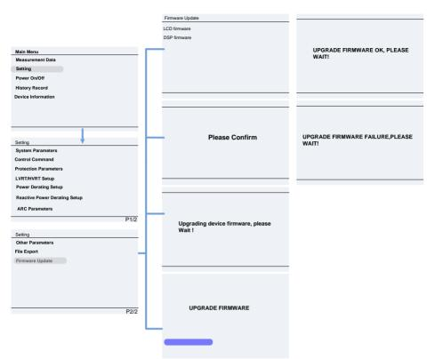
Figure 6.7 – Firmware Upgrade Interface
