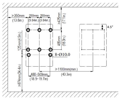
Figure 2.5 - Holes on the Bearing Surface Dimensions
