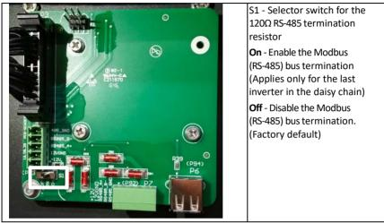
Figure 2.46 - The Modbus (RS-485) Termination Switch (S1) Location and Settings on the LCD/Communication Board.
