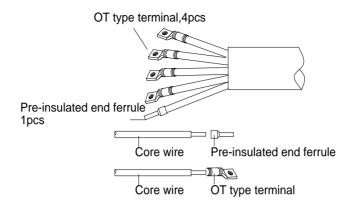
Figure 2.37 - AC Output and Ground Cable Setup
