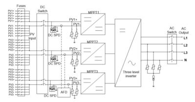
Figure 1.2 - Schematic Diagram of PVI 50/60TL Inverter
