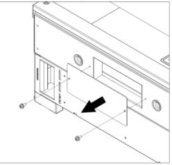
Figure 2.10 – Main Section Cover Plate
