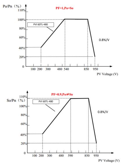
Figure 7.2 - PVI 60TL kW and kVA Derating Curves of PV Input Voltage
