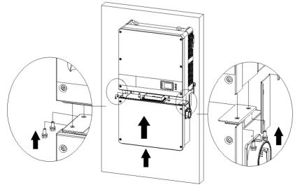
Figure 2.12 - Wiring Box Installation
