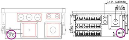
Figure 2.38 - External Chassis Ground
