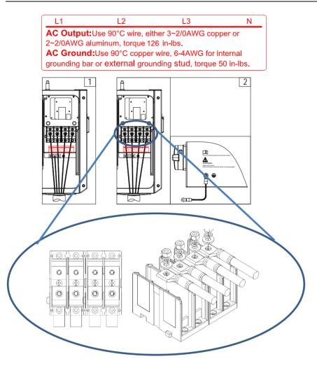
Figure 2.36 - AC Output and Ground Cable Connections
