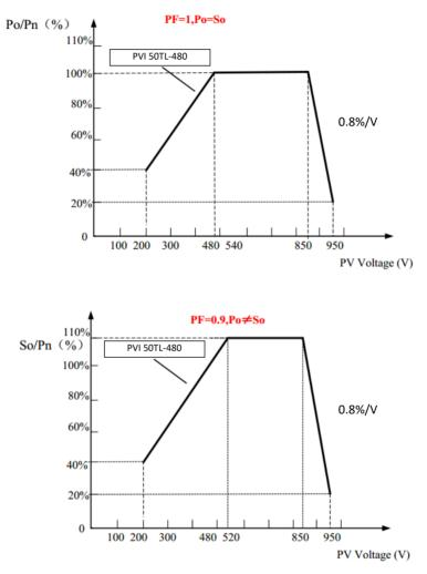
Figure 7.1 - PVI 50TL kW and kVA Derating Curves of PV Input Voltage
