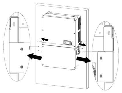
Figure 6.3 - Remove the Screws on Both Sides
