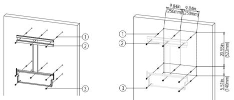
Figure 2.7 - Securing Mounting Bracket
