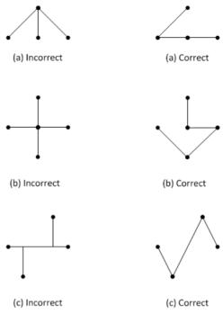
Figure 2.45 - Correct and incorrect topologies
