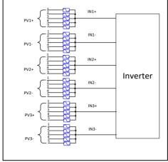
Figure 2.33 - Three MPPTs Operating Independently
