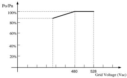
Figure 7.5 - PVI 50/60TL Derating Curve of Grid Voltage
