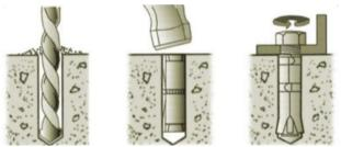
Figure 2.6 – Drilling holes for mounting hardware
