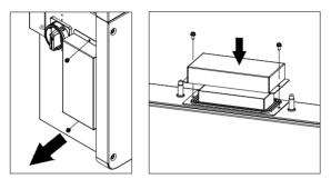
Figure 6.5 - Install the Cover Board on the Connector of the Wiring Box
