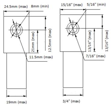
Figure 2.35 - AC Cables' Crimp Lug Specification (a) Standard (b) Metric
