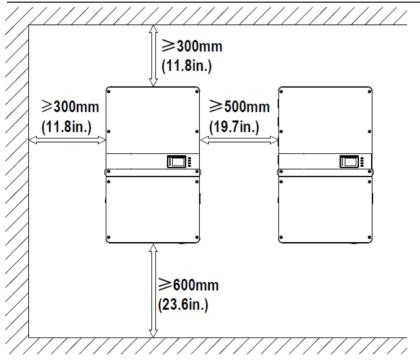
Figure 2.3 - Inverter Wall Mounting Specifications
