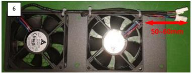
Figure 6.1 - Replace Cooling Fans
