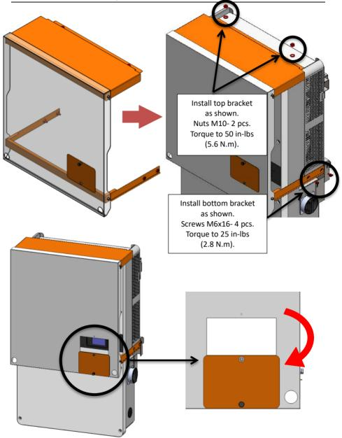
Figure 8.4 – Shade Cover Installation; Steps 3 and 4
