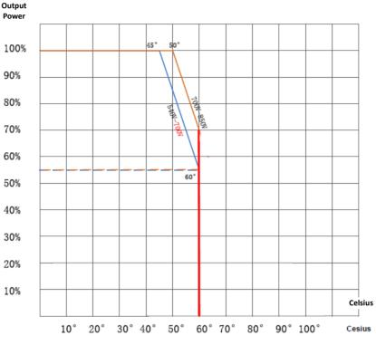
**NOTE 2:** When the ambient temperature is higher than 113°F (45°C), the output power may begin derating. For DC voltage as shown in Figure 7.3:
