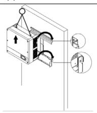
Figure 2.8 - Mounting the Main Inverter Section on the Bracket
