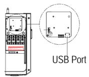
Figure 6.6 – USB Port for Firmware Upgrades
