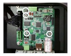
Figure 2.48 - Ethernet Network Card Installed
