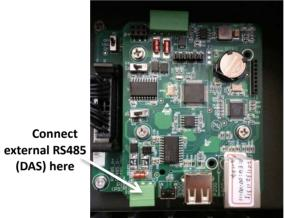
Figure 2.49 - Ethernet Network Wiring to DAS 2.4.8 Preparing the Ethernet Network Card
