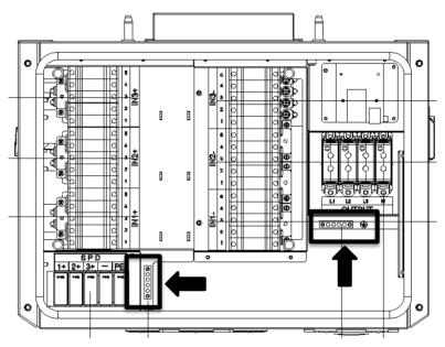
Figure 2.24 - Equipment Grounding Locations (Standard Wiring Box)
