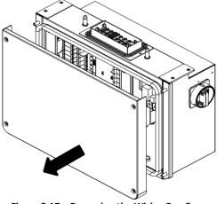
Figure 2.17 – Removing the Wiring Box Cover
